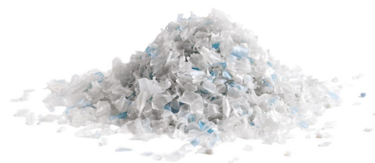
1 Plastic bottles are shredded into flakes.
