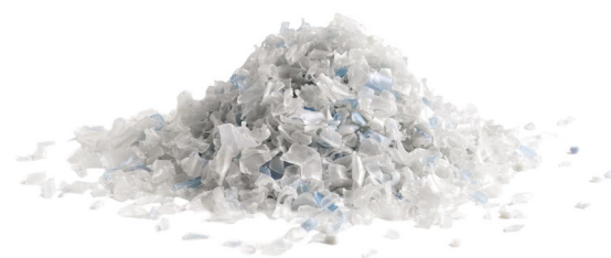
1 Plastic bottles are shredded into flakes.
